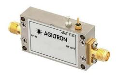
This is a high-gain, low-noise 2-stage amplifier delivering 3.3 Vp-p output across a broad frequency range of 30 kHz to 45 GHz. It is a general-purpose broadband driver amplifier optimized for Mach-Zehnder optical modulator applications, offering low power dissipation, high drive capability, very low added jitter, and fast rise time. The amplifier requires a 12 V DC power supply at 1W and features a GPPO male connector. A compatible power supply is included for user convenience.
